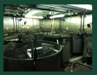
Respirometry chambers measure O<sub>2</sub> consumption over 24hrs
