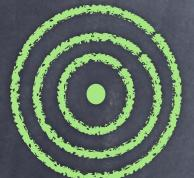
if there is a hole in the screen and its diameter matches the diameter of the airy disk most of the intensity will pass through it to the PMT detector
